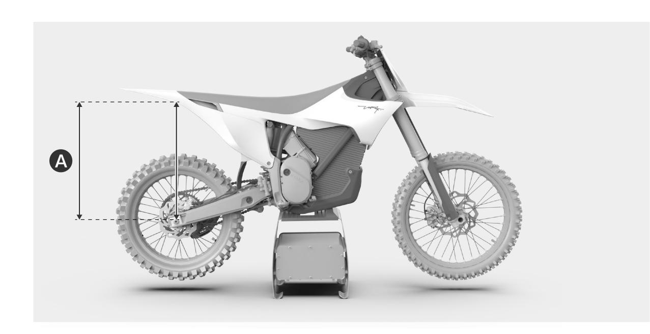
1 Measure the height A between the wheel axle and the SAG marking on the rear spoiler with the bike on the stand and both wheels off the ground.
