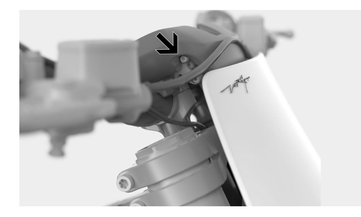
2 Press down the docking station release lever and take out the phone.
