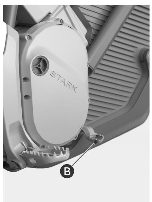
A Front hand brake B Rear brake tip
