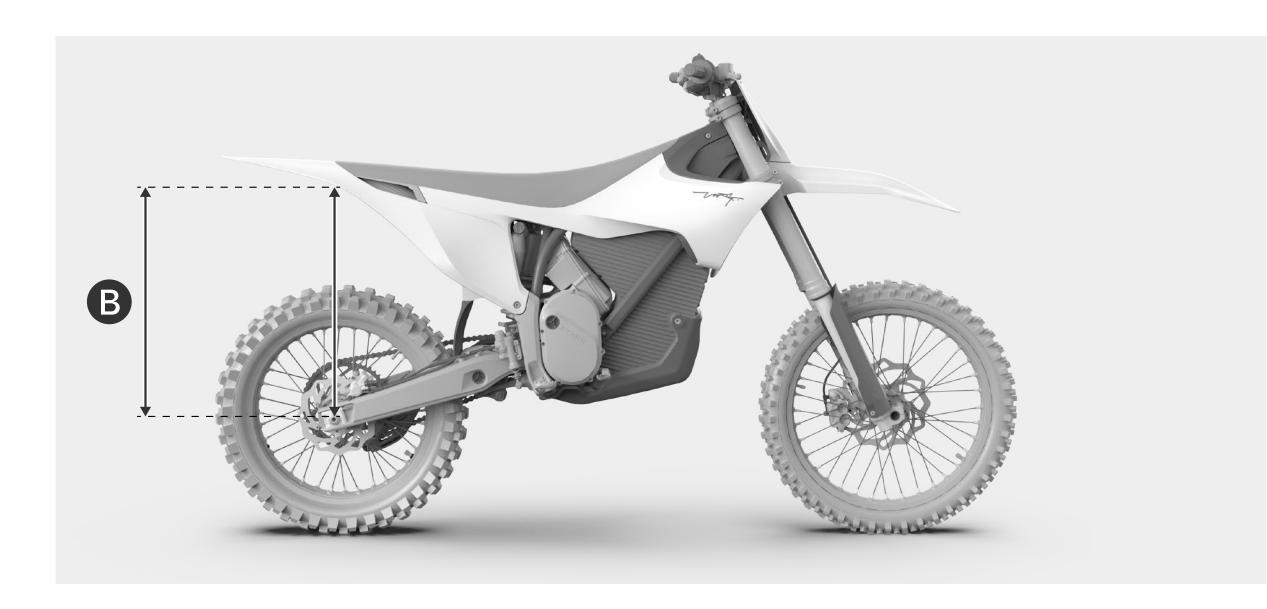
2 Place the bike with both wheels on the ground and measure the **height B** between the wheel axle and the SAG marking on the rear spoiler. Recommended value is: **height A** (see step 1) 40 mm +/- 3 mm.
