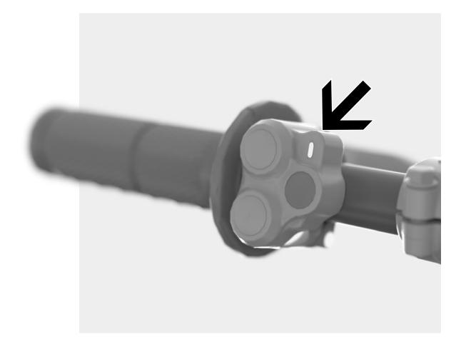
The control switch contains a **LED light** which can change color.
