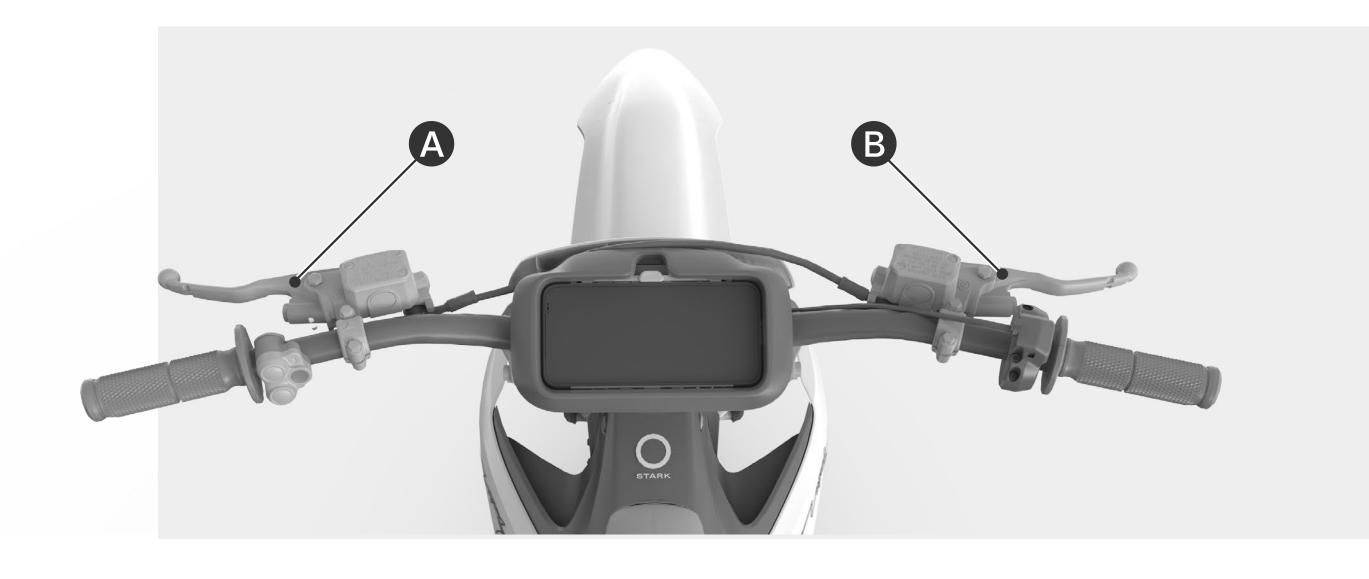
A Rear hand brake B Front hand brake
