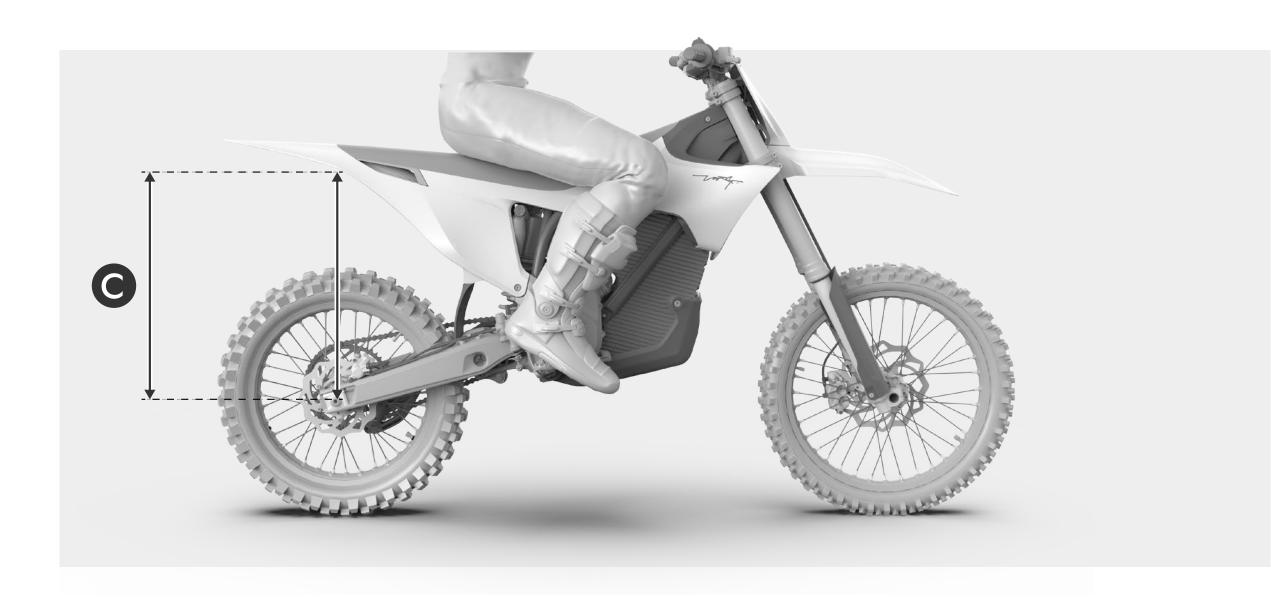
3 Place the bike with both wheels on the ground and, with a rider sitting on the bike, measure the height C between the wheel axle and the SAG marking on the rear spoiler. Recommended value is: height A (see step 1) 110mm +/-3mm.
